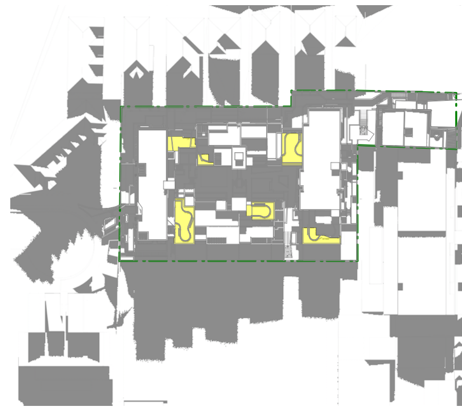
09:30 AM area of PUCOS receiving sun 375.2 sq m percentage of total PUCOS 55.2%
