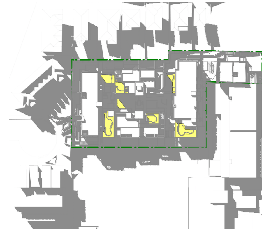
12:00 PM area of PUCOS receiving sun 367.1 sq m percentage of total PUCOS 54%
