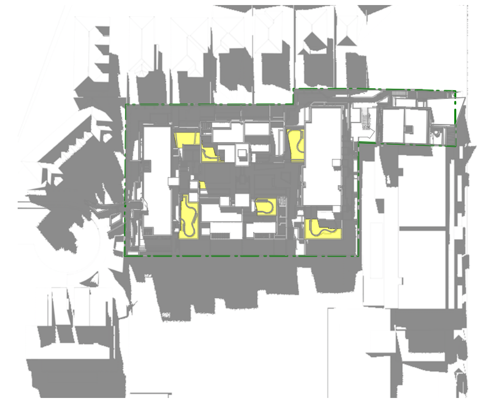
10:30 AM area of PUCOS receiving sun 377.7 sq m percentage of total PUCOS 55.6%
